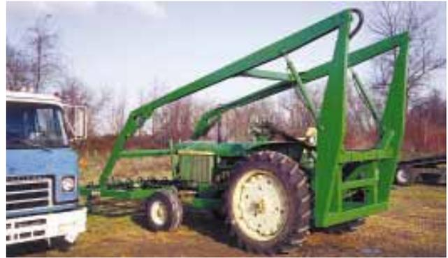
Loader's steel frame bolts to underside of tractor and a pair of big steel arms attach to 3-pt. hitch. Loader is shown here mounted on a Deere 3010.
