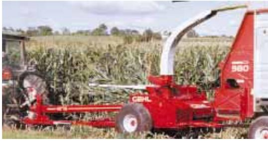
Gehl's new 1275 forage harvester cracks the entire kernel, breaks up cobs, and "conditions" stalks, producing higher value silage.
