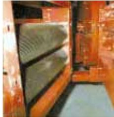
Two high speed 1/2-in. dia. rollers mount directly behind cutterhead cylinder.
