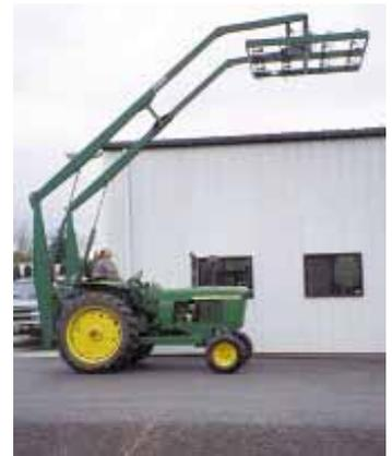
Arms extend out over front of tractor and are raised or lowered by a pair of hydraulic cylinders.
