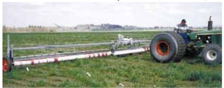
Wiper uses nozzles to spray foam concentrate onto a rotating roller which wipes the foam chemical solution on weeds. Note streaks on roller where weeds rubbed foam off.
