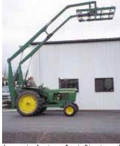
Arms extend out over front of tractor and are raised or lowered by a pair of hydraulic cylinders.
