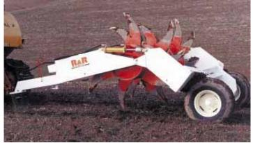
Rig is equipped with 18 shanks mounted on a rotary drum that are arranged in an overlapping design. Penetrates to 24 in. deep with minimal topsoil disturbance.
