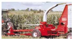
Gehl's new 1275 forage harvester cracks the entire kernel, breaks up cobs, and "conditions" stalks, producing higher value silage.
