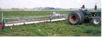
Wiper uses nozzles to spray foam concentrate onto a rotating roller which wipes the foam chemical solution on weeds. Note streaks on roller where weeds rubbed foam off.
