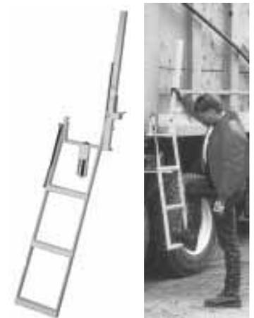
Ladder comes with 36-in. high grab handle. Steps flip up and latch to handle when not in use.
