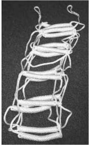
Entire ladder is made from a single length of 3/8-in. dia. nylon rope. Its light weight makes it easy to carry around.
