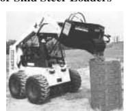
"Mud Bucket" lets one person accurately place concrete into forms with no need to
