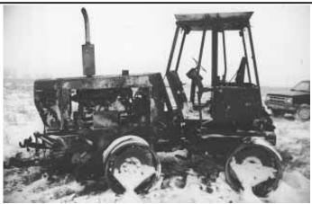
Insurance investigators believe the fire that destroyed this Ford-New Holland bidirectional tractor started in the wiring.
