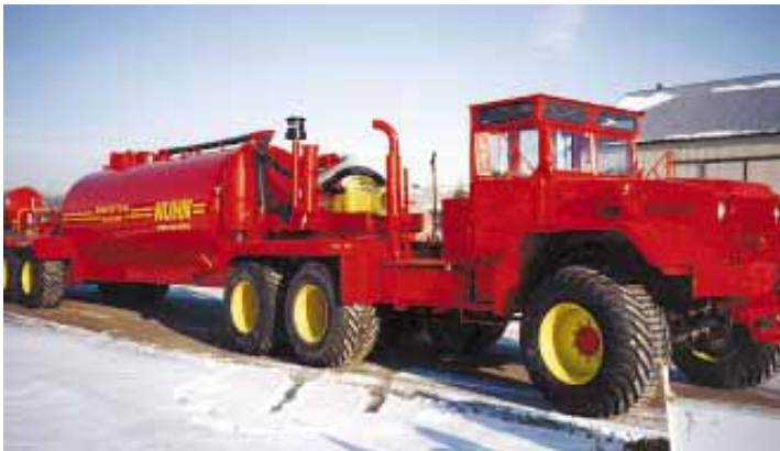
Nuhn Industries removed the bed from this used 6-WD Army truck and added a fifth wheel hitch and trailer, then installed a 24-ft. long, 6,750-gal. liquid manure tank.
