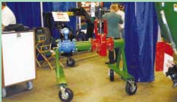
Flow meter and pinch valve precisely vary rates on-the-go. System installs between the discharge and injectors on liquid manure tanks.
