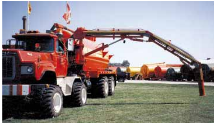
A 40-ft. long, 8-in. dia. self-loading boom mounts on driver's side. Hydraulic-controlled boom allows operator to use push button controls in cab to fill tank from a pit.
