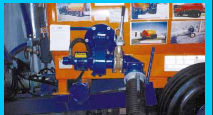
Hydraulic-driven impeller installs in wagon's vacuum suction line to help speed up fill time. Unit is designed for 4,000-gal. and larger wagons.
