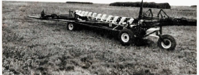
Melius equipped his 13 bottom plow with a rear hydraulic marker that raises and lowers with the plow’s rear wheel.
