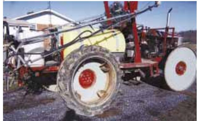
Sprayer can be fitted with these special-built rubber tire wheels whenever the ground is wet.
