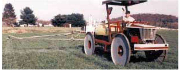
Rig is equipped with 2 1/2-in. wide steel wheels faced with hard rubber. The narrow wheels allow it to work in solid-seeded standing crops without doing damage.
