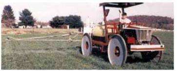
Rig is equipped with 2 1/2-in. wide steel wheels faced with hard rubber. The narrow wheels allow it to work in solid-seeded standing crops without doing damage.
