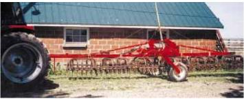
To attach hoe to carrier, Martin backs the carrier over the hoe and uses planter's original hydraulic lift cylinder to lower unit down over hoe. He then hooks up the chains.
