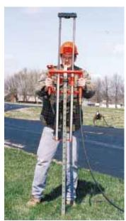
Post driver's 26-in. long ram is triggered automatically as you set the unit onto the top of the post. Unit weighs only 39 lbs.
