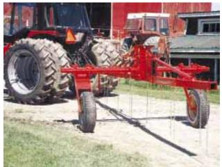
Lengths of chain welded onto opposite sides of square steel bar running lengthwise are used to attach hoe to carrier.
