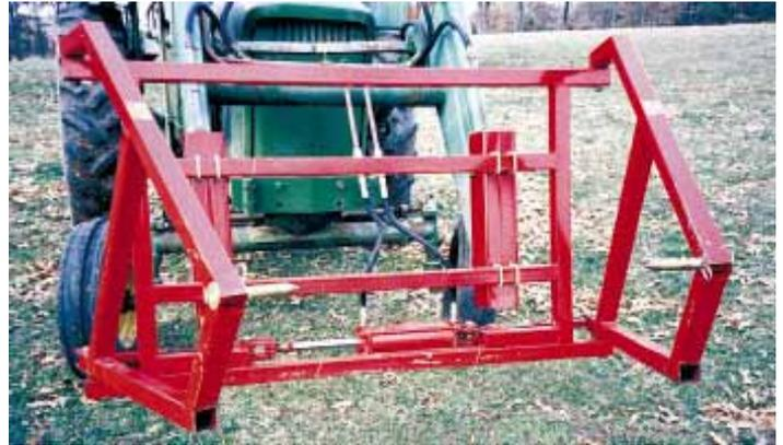
"Hay Hand" uses a pair of hinged frames to grab bales. A short spear on each side helps hold bale in place. Arms are opened or closed by a single hydraulic cylinder.
