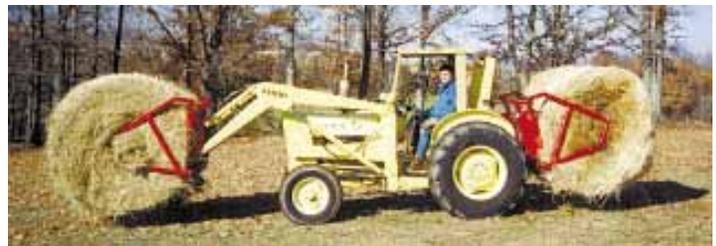
Unit can be mounted on a front-end loader or 3-pt. hitch.
