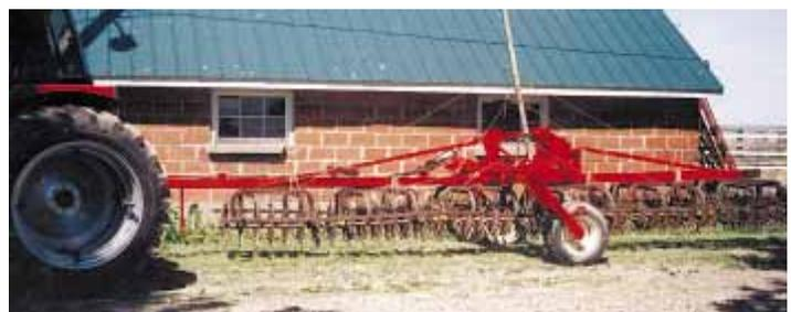
To attach hoe to carrier, Martin backs the carrier over the hoe and uses planter's original hydraulic lift cylinder to lower unit down over hoe. He then hooks up the chains.
