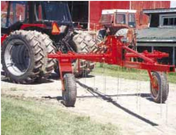
Lengths of chain welded onto opposite sides of square steel bar running lengthwise are used to attach hoe to carrier.
