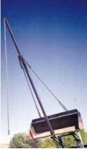
The 15-ft. long boom mounts on loader bucket to extend its lifting ability, in effect creating a miniature crane.
