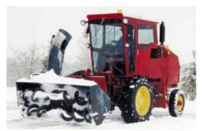
Self-propelled rig is shown here equipped with a 7-ft. wide double auger blower that's driven by a 4-speed truck transmission.
