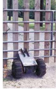
"Remote control" opener bolts directly to a 16-ft. steel gate across McCaslin's driveway, allowing him to open and close the gate right from his vehicle.
