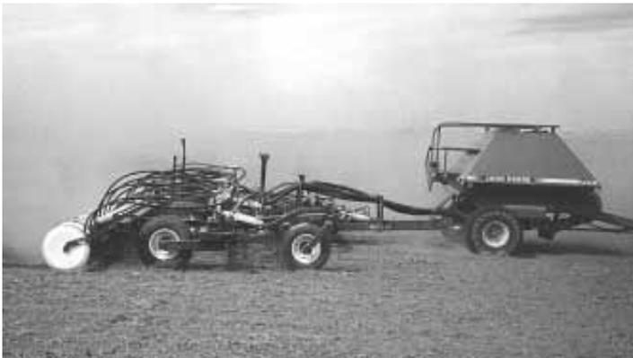
New 36-ft. wide air seeder features a 3-section frame that flexes on even the hilliest ground.
