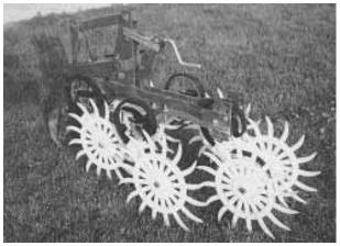
A standard 20-in. dia. rotary hoe wheel runs between every cultivator shovel
