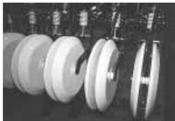
Split packer wheels provide individual depth control for accurate placement.
