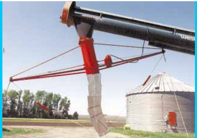
Winch-operated cable pulls auger spout to either side. A rope attached to each end of cross arm allows Lindhorst to line up unit with the truck or wagon.
