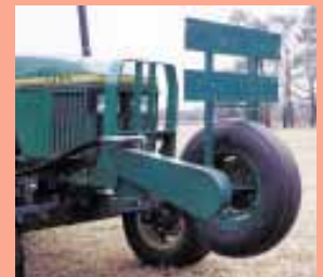
A channel iron frame bolts to weight bracket on front of tractor.
