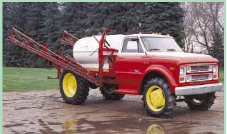
Wahouske fitted a 1972 Chevy 1 1/2-ton truck with a 650-gal. tank and 90-ft. rear-mounted manual-fold boom. The 30-in. rear wheels are off a Deere MFWD tractor. The 22-in. front wheels are off a Deere utility tractor.
