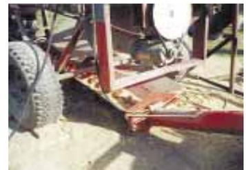
Powered by an orbit motor, the system is usually operated every load or two.
