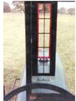
Red frame should be seen just inside the black screen on cab window.
