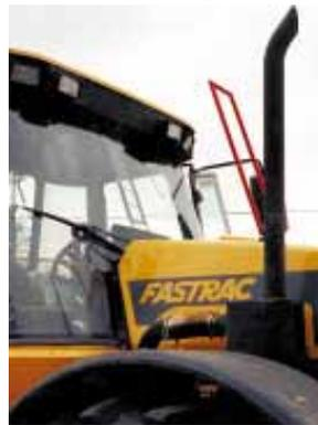
"Eyesite" mounted parallel to windshield on Fastrac tractor.
