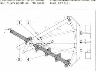
By activating the hydraulic ram, the toolbar is swung to the left or right around the pivot point. The front end of the toolbar runs on rollers along the curved rail, the extremeties of which produce an operating angle of up to  $45^\circ$ .
