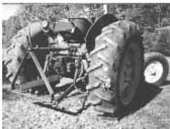
I bent a piece of 1/4 by 2-in. scrap iron into an inverted V shape with a flattened apex. I torched a 3/4-in. dia. hole in the flat to accept a Cat # 1 pin and welded the free ends to the drawbar. I welded two balls and a pin to accept a pintle hitch to the bar. Pinned in the top, it has enough movement to prevent bending and raises and lowers on the lift arms almost perfectly."
