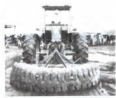
After seeing a 3-pt. scraper in FARM SHOW some time back, I decided to build my own using a giant industrial tire. I cut the tire in half and bolted it to a 3-pt. mounted frame. The tire does a great job scraping manure off feedlots. Doesn't wear down the concrete and moves wet manure better than a blade. (Matt Luce, Rt. 12, Rockwood, Penn. 15557)
