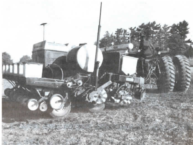
Add-on front toolbar carries dry fertilizer hoppers and no-till attachments.
