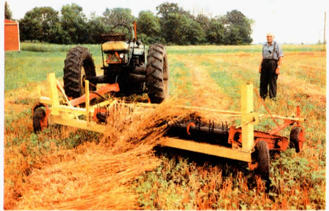
You can set the windrow on the same strip or move it over 3 ft.
