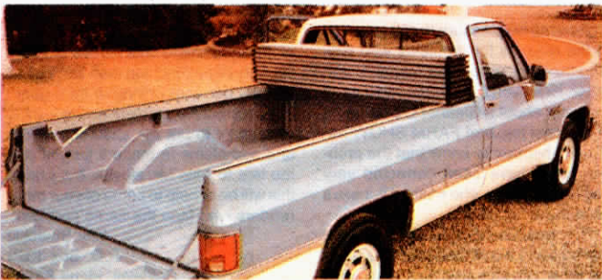
Aluminum slats (10 in. wide) accordion-fold into a single stack behind the cab when not in use.
