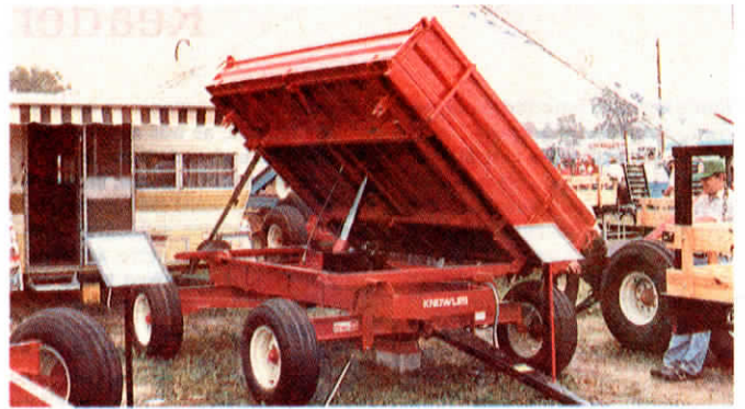
A pair of lock pins determines whether box dumps right, left, or backwards.
