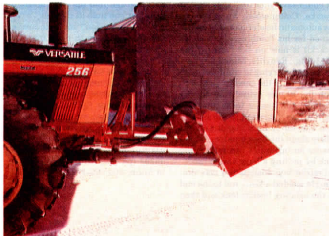
Vacuum tube, fastened to a galvanized metal pipe, attaches to rear of loader bucket.
