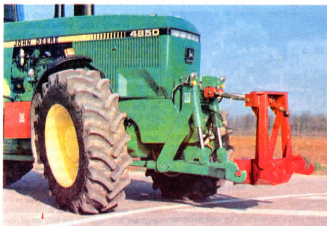
Deere 4850 equipped with Laforge front 3-pt., depth control, weight transfer module and interface connection (in red) to follow ground contour. Brace under tractor runs from front 3-pt. to rear drawbar.
