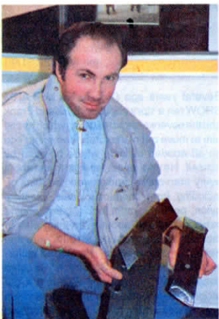
Paul Pumfrey holds reversible replacement point which is secured to plow share with two bolts.
