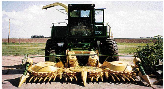
Machine is fitted with a 6-row Kemper head powered by a 20 gpm hydraulic pump.
