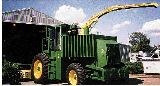
A 50-gal. capacity radiator mounts on back of chopper. A hydraulically-driven 36-in. dia. fan blows air out rear of machine, moving heat and noise away from driver.
