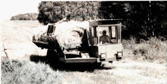
The 32-ft. long machine carries 12 5-ft. bales and has a top speed of 50 mph.
