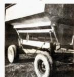
allow it to hinge enough to dump. He says on other, differently designed wagons it would simply be a matter of building heavy hinges and welding them in place. Once modified, he says it's not necessary to pin down the unbolted side of the wagon. The weight of the box keeps it in place.
