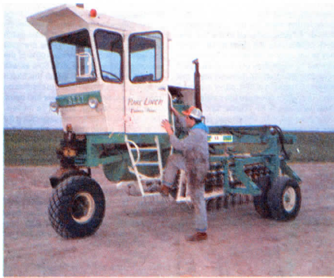
The self-propelled rake is equipped with an up-front cab and a Pontiac V-6 engine.
