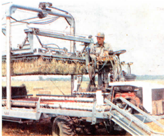
As bales are retrieved from field, they're arranged in layers by powered rollers. Each completed layer is picked up by an overhead clamp and loaded onto a pallet at rear.
