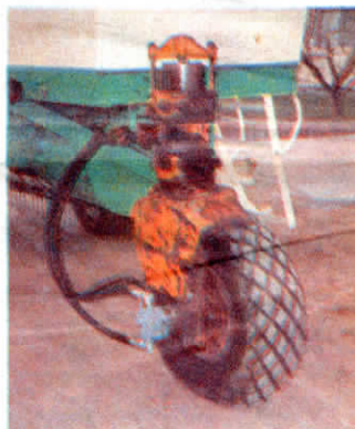
The rake's single drive wheel is driven and steered hydraulically.
