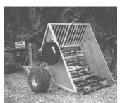
Feeder tips backward for loading. Handcranked winch on front is used to load
