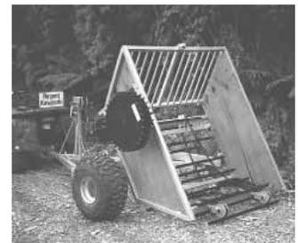
Feeder tips backward for loading. Hand-cranked winch on front is used to load bale.
