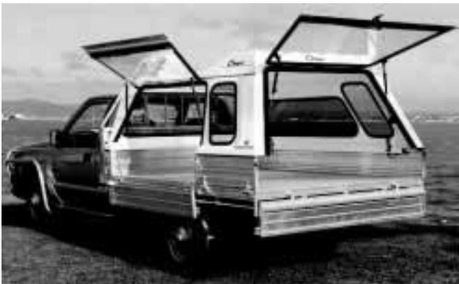
Side-opening topper fits special-built deck with fold-down, 1-ft. high sides.
