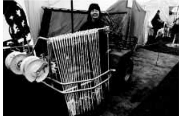
Detachable aluminum frame can carry two wire reels and up to 26 posts.
