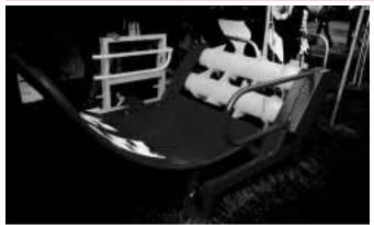
Extending a cylinder raises curved steel cradle which feeds bale into beaters.
