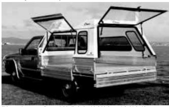
Side-opening topper fits special-built deck with fold-down, 1-ft. high sides.
