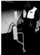
Feeder uses a shot of compressed air to loosen soil around tree, allowing roots to grow more freely.
