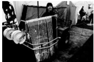
Detachable aluminum frame can carry two wire reels and up to 26 posts.
