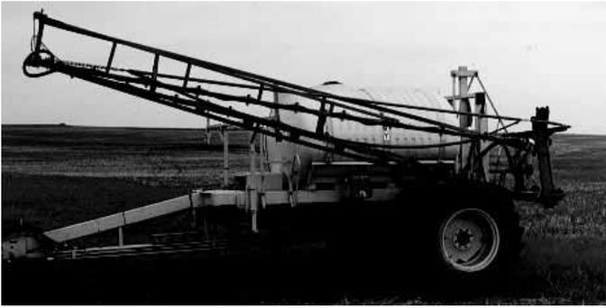
Sprayer's axle came off an old Deere 96 pull-type combine and tires off a Deere front wheel assist tractor. Henry used 4 by 6-in. steel tubing to build sprayer frame.
