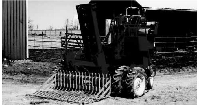
Seymour fitted swather with a heavy-duty mast off a junked forklift. He uses the lift to pick rocks by mounting a commercial rock picker bucket on front.
