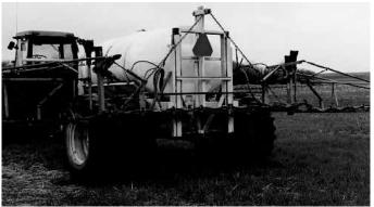
Using duals on both tractor and sprayer leaves a light footprint. Slide assembly on back allows booms to be hydraulically raised or lowered 3 ft. depending on crop height.
