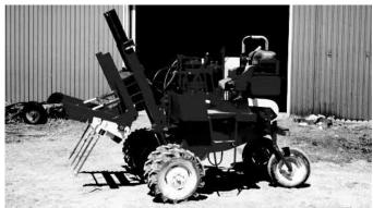
To lift bales Seymour built a quick-tach bale fork fitted with four 27-in. long prongs.
