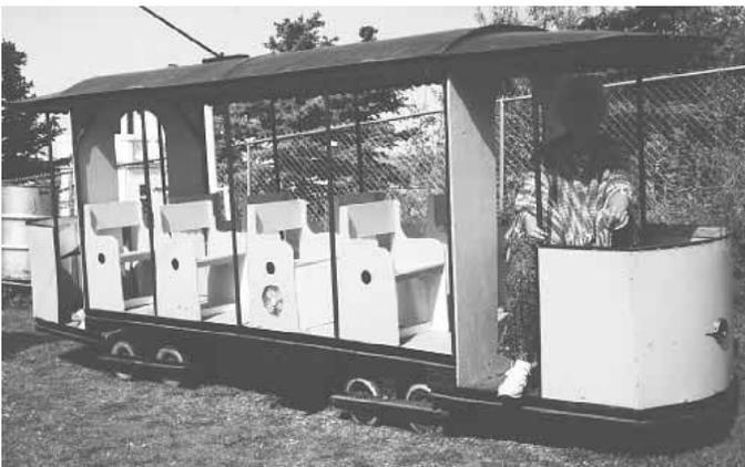
Rogers' street car is powered with an 8 hp vertical Briggs and Stratton engine mounted under the second seat.
