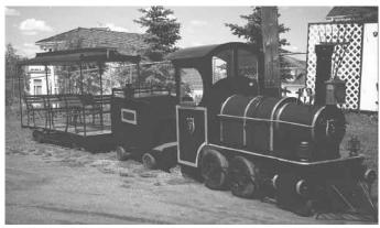
Rogers' locomotive is powered by a 12 hp heavy-duty Wisconsin gas engine connected to an automotive transmission providing four forward speeds and one reverse speed.
