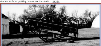
Two 16-in. wide, 20-ft. long ramps mount on 40-in. high V-shaped "rocker" frame.
