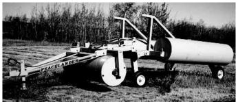
The 40-ft. roller is built in three sections equipped with 42-in. dia. drums.
