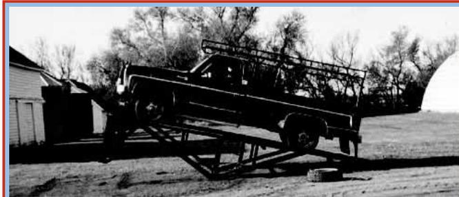
Two 16-in. wide, 20-ft. long ramps mount on 40-in. high V-shaped “rocker” frame.
