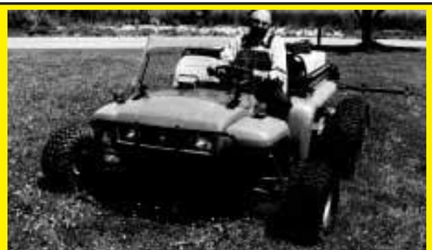
Burt widened out “Gator” wheelbase to 76 in. because he plants in 38-in. rows. Front wheel supports were widened and the rear end was completely rebuilt.
