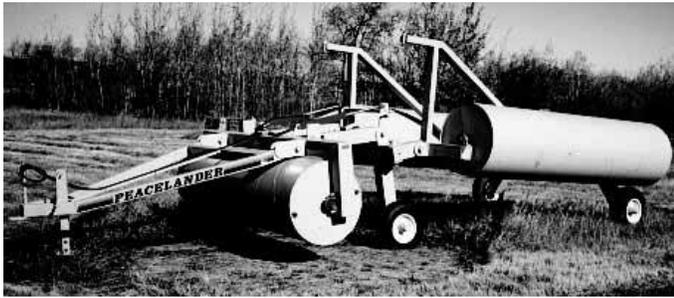
The 40-ft. roller is built in three sections equipped with 42-in. dia. drums.
