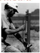
An inner sleeve clamps in place. Air pressure lifts the device off the sleeve, then drives it downward at a rate of 80 to 85 strokes per minute.
