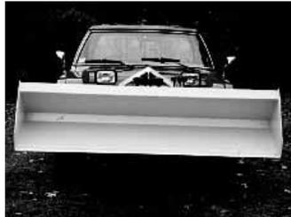
Bucket is about 4 ft. wider than pickup wheels and has a capacity of just under two yards.
