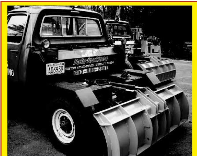
CCS also builds a shortened up version of a 4-WD pickup equipped with the "pull plow" blade as well as an 80-gal. fuel tank on back. The blade mounts tight up against the back of the pickup. Works great to remove snow in an enclosed area or next to a garage door or wall, etc. You simply back up to a wall, drop both blades, and drive forward. Because you're pulling snow, you never have to turn the pickup around in order to "back drag" snow.
