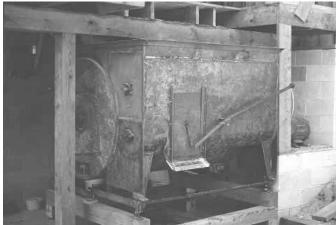
the housing for the unloading auger. I mounted the mixer on wooden blocks so I can load directly into my wheelbarrow without the need for an elevator.
