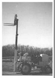
filled the combine hood with 1,200 lbs. of concrete and mounted it on the rear too. That did the trick."
