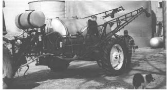
sprayer with a 2-in. dia. suction line from the bottom of the tank to the pump and a 11/2-in. dia. return line.
