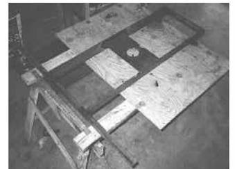
**Acme gearbox mounts on plate that mounts on lateral braces.**
