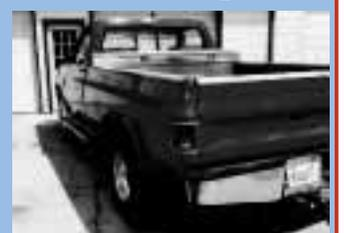
In order to mount duals on the 3/4-ton pickup Brittin replaced the original axle with a 1-ton Chevy axle.
