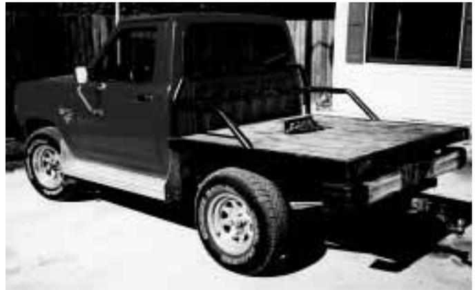
Brittin cut off the back part of a wrecked Ford Bronco, attached part of a Ford Ranger pickup cab, and added his own remote-controlled hydraulic tilt bed.
