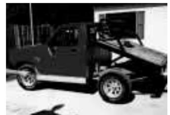
Brittin uses a remote control button on his key chain to tilt the bed up or down.
