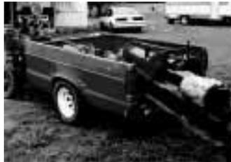
Engine’s driveshaft belt-drives the pickup transmission. Homemade cylinder applies 50,000 lbs. of force.
