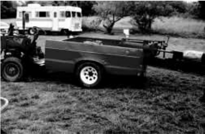
Splitter mounts on cut-off pickup bed pulled by a 40 hp Wisconsin engine.
