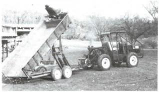
The log skidder bends in the middle by means of a pair of 2 1/4-in. dia. hydraulic cylinders that act on a 2 1/2-in. dia., 14-in. long kingpin.
