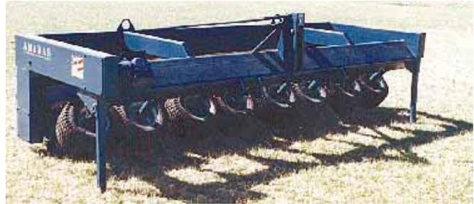
Chopper uses spinning rubber tires to pull stalks out by the roots and then chops them up with a drum-type chopper that follows behind.
