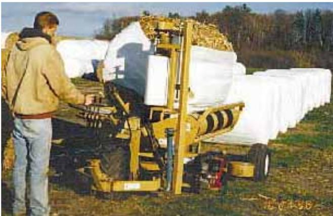
Operator walks in front using control levers mounted on the steering arm. Note big drive wheel which is chain-driven by an orbit motor.
